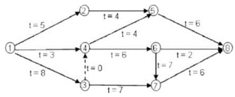
A construction company has to submit a bid for the construction of a new apartment building. The PERT network along with the three time estimate (in week) for each activity of the project is shown in the figure below. Determine critical path and its standard deviation. Probability of completing the work in 34 weeks
