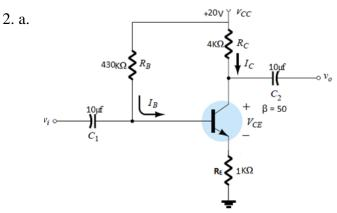
For the emitter bias network of Fig., determine
