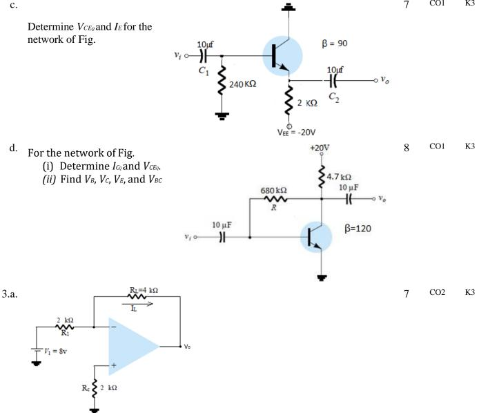
For the circuit of Fig. calculate  $I_L \& V_0$
