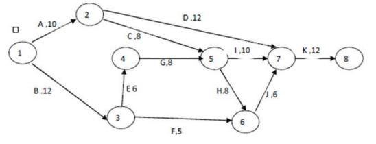
Also find the Total float, Free float, Independent float and Interfering float for each activity.
