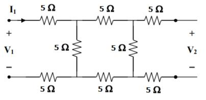
b. For the circuit shown in figure, the resistance of  $5\Omega$  changes to  $2\Omega$ . Calculate 7 CO1 3 the compensation source and verify the results.
