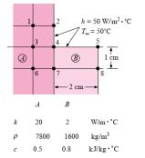
5. Write the transient nodal equation for node 7 in Figure. Physical and thermal properties (6) of materials *A* and *B*are shown in the figure.
