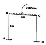
5. Draw shear force and bending moment diagram for the beam given in Fig.
