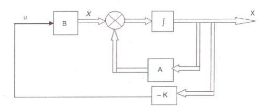
The system uses the state feedback control U=-kX. If the desired closed-loop poles are located at s=-2+j4, s=-2-j4, s=-10. Determine the state feedback gain matrix K using any two methods.
