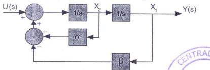
Obtain the state model of the system and determine the eigen values of the system.
