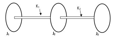
$K_1=0.10 \times 10^6$  Nm/rad,  $K_2=0.20 \times 10^6$  Nm/rad  $J_1=5.0$  kg.m<sup>2</sup>,  $J_2=11.0$  kg.m<sup>2</sup>,  $J_3=22.0$  kg.m<sup>2</sup>
