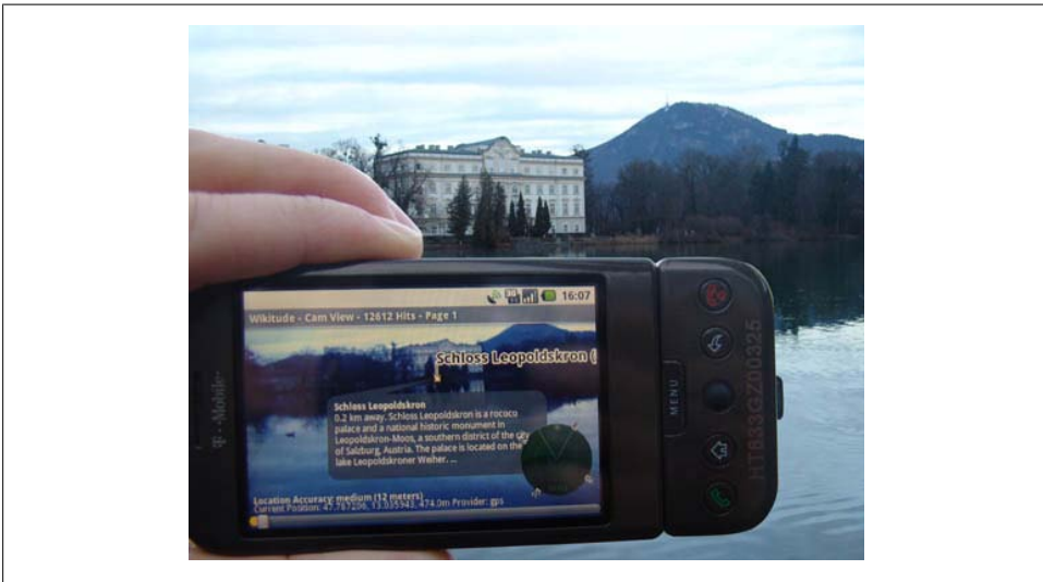
Figure 4-9. The Android application Wikitude presenting information from the Web in the context the user's present location
