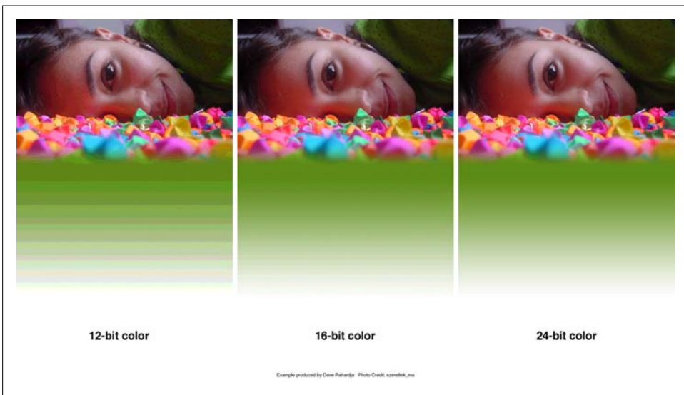
Figure 8-10. An example of different levels of posterization that can occur across multiple device color depths
