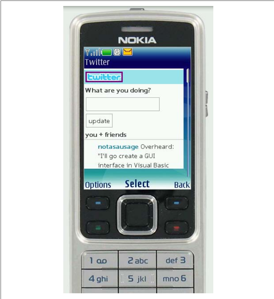
Figure 8-9. Example layout of a scroll-based application, where the user had to press the D-pad past each link to scroll the page
