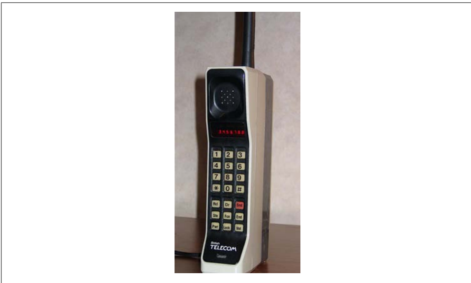
Figure 1-3. The Motorola DynaTAC 8000X was the first mobile phone to receive FCC acceptance, in 1983; DynaTAC was actually an abbreviation of Dynamic Adaptive Total Area Coverage
