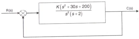
Using Routh-Hurwitz criterion, determine the range of K for which the system is stable. Find also the number of roots of the characteristic equation that are in the right half of the s-plane for K=0.5.
