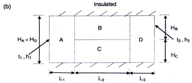
A composite wall having unit length normal to the plane of paper is insulated at the top and bottom as shown in figure. It is composed of four different materials A,B,C,D. The dimension of are  $H_A = H_D = 3$  m,  $H_B = H_C = 1.5$  m,  $L_1 = L_3 = 0.05 \text{ m}, L_2 = 0.1 \text{ m}$
