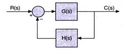
Show that the system is unstable for all positive values of the gain K. This system can be stabilized by adding a zero on the negative real axis to modify G(s) to
