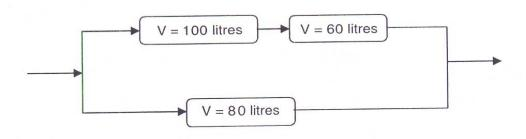
An aqueous feed of A and B (400 litre/min, 100 mmol A/litre, 200 mmol B/litre) is to be converted to product in a plug flow reactor. The kinetics of the reaction is represented by
