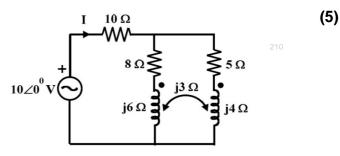
**Q5**<sub>0</sub> **a)** Find Z parameters of the two port network.
