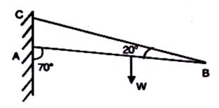
(b) A rigid prismatic bar 5m long is supported in a vertical plane by hinge at one end and by a horizontal string attached to it at its mid-point. A 150N weight
