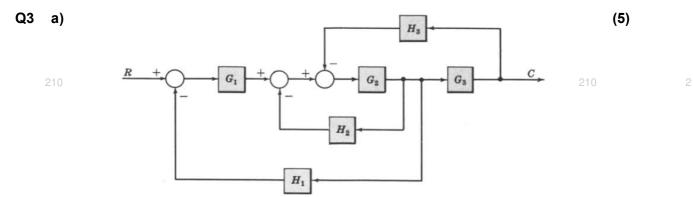
Find the transfer function C/R using block diagram reduction techniques.
