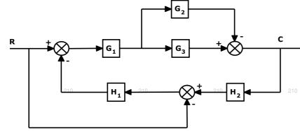
Determine the transfer function(C/R) of the system shown in Fig, using Mason's Gain Formula.
