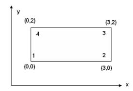
Take  $E=2x10^5$  N/mm<sup>2</sup>, poission ratio v = 0.25. Assume plane stress condition. The displacements of nodes 1, 2, 3 and 4 in x-direction 0,0.002,0.005,0 and in y-direction 0,0.003,0.003,0 mm respectively.
